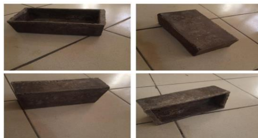
Plate 3. Composite Mould of rLDPE and Sawdust (different views)
