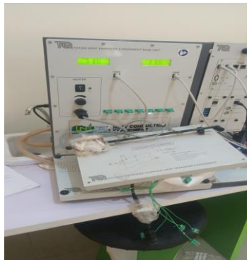
Plate 5. TecQuipment (TQ) TD 1002 thermal conductivity experiment carried out
