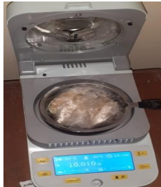
Plate 4. BIOBASE infrared moisture analyzer loaded with sample
